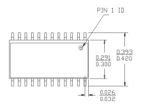
DIMENSIONS IN INCHES MIN. MAX. LEAD COPLANARITY 0.004 MAX.
