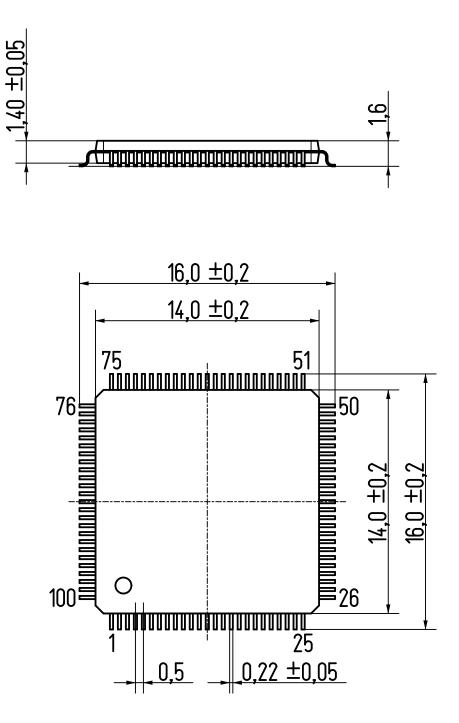
Package thickness: 1.4 mm ±0.05 mm All dimensions: mm
